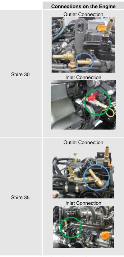
Figure 16: Calorifier Connections
