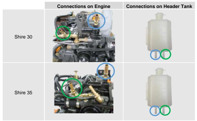
Figure 11: Header Tank Connections
