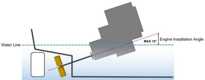
Figure 15: Maximum Engine Installation Angle
