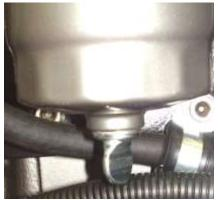
Figure 19: Primary Fuel Filter Drain Screw
