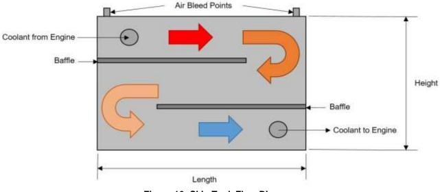
Figure 10: Skin Tank Flow Diagram
