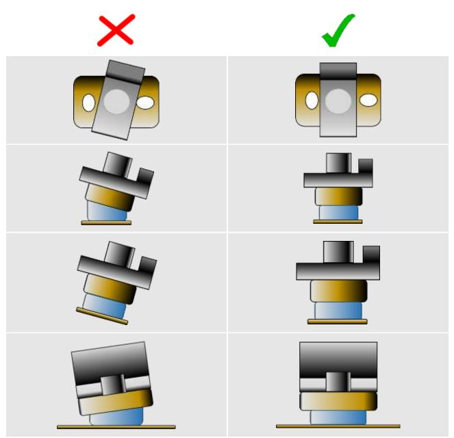
Figure 12: Correct Anti-Vibration Mount Installation
