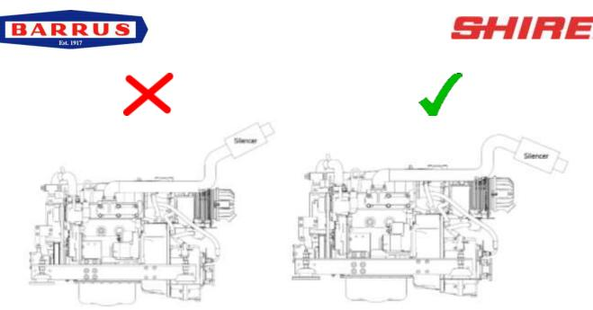
Figure 17: Correct Exhaust Installation
