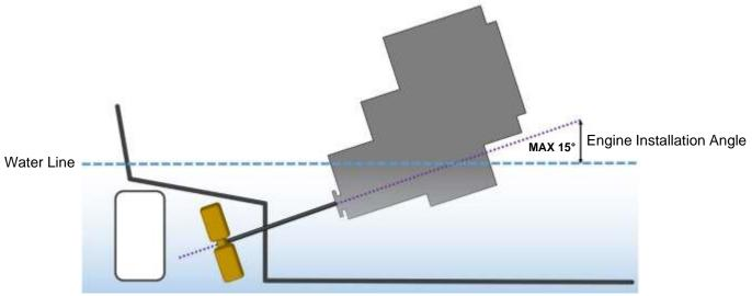
Figure 22: Maximum Engine Installation Angle
