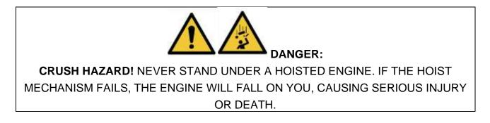
The Lifting points supplied with the engine are for lifting the engine/gearbox only. A suitable spreader bar must be employed to prevent over-stressing either bracket during any lift.
