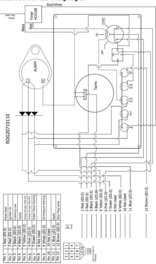
Figure 28: Standard Control Panel Wiring Diagram
