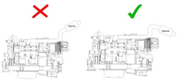
Figure 23: Correct Exhaust Installation
