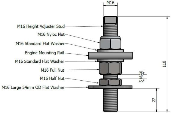
Figure 20: Correct Anti-Vibration Mount Installation
