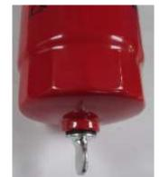
Figure 26: Primary Fuel Filter Drain Screw
