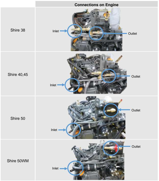
Figure 18: Calorifier Connections
