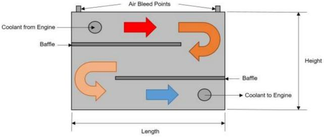
Figure 16: Skin Tank Flow Diagram
