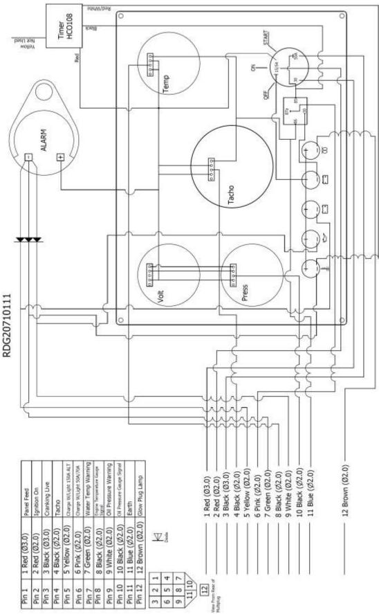
Figure 29: Deluxe Control Panel Wiring Diagram
