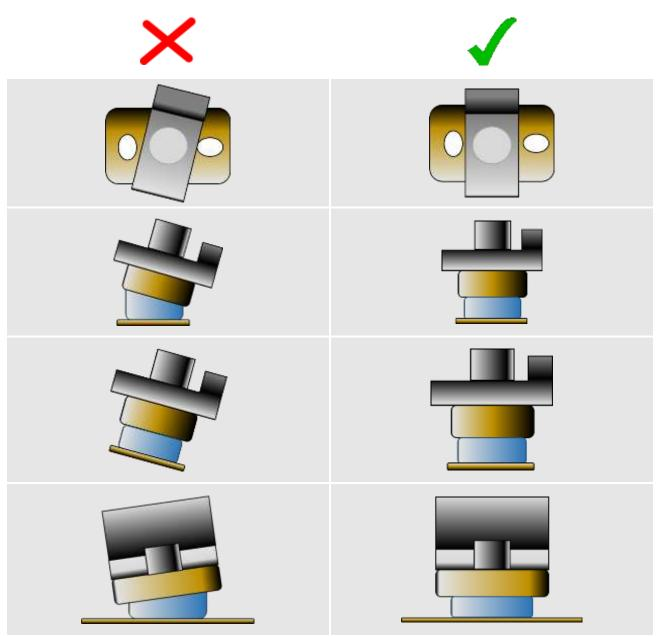
Figure 19: Correct Anti-Vibration Mount Installation
